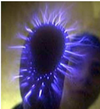
Figure 1. The discharge created around a fingertip, recorded in original natural colours [20]. View from underneath, through a semi-transparent glass electrode that provided electrical field excitation. Remark: Figure 1 in the Internet version of the journal is presented in colour.
